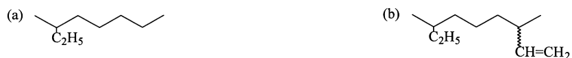
Fig. 1. Structural formulas of examined materials: (a) ethylene with butene as comonomer; and (b) ethylene copolymerised with butene and 1,9-decadiene.
